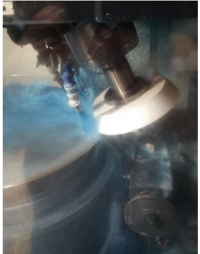
Face grinding a ring gear with an angle head wheel
