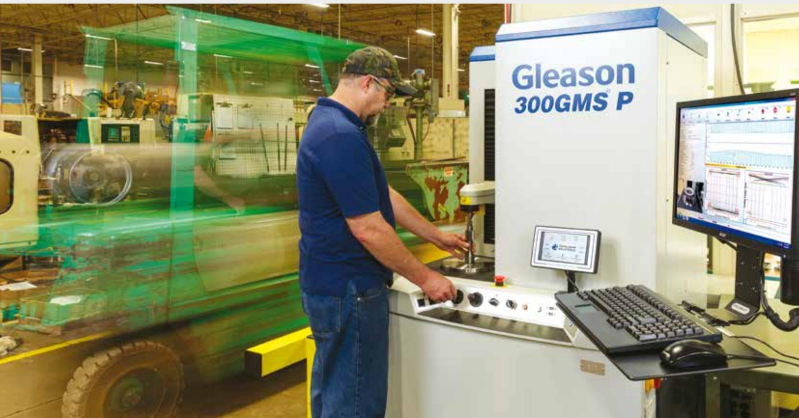
Putting a 'shop-hardened' 300GMS®P in close proximity to Schafer's two high-volume hard finish grinding cells saves hours of queue and transport time every day. Vibration from forklifts and nearby shaping operations, as well as temperature changes, have had no impact on the system's ability to deliver exceptional inspection results.
