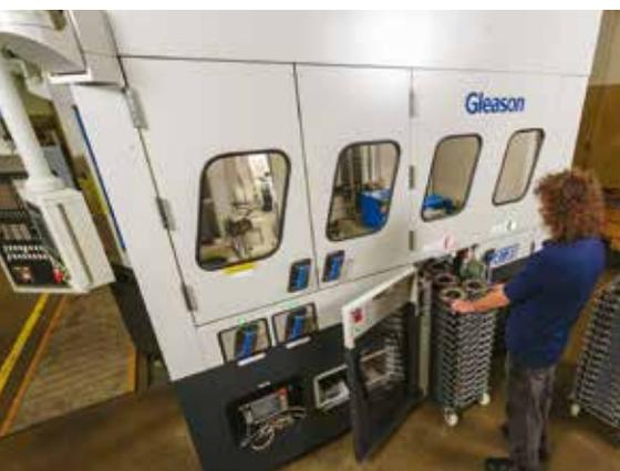
Integration of a Gleason Automation Systems' modular Machine Tool Loader puts 180 parts in stackable trays ready for robot load. This is up to 6 times the number of unattended parts in the queue as compared to a traditional conveyor system.
