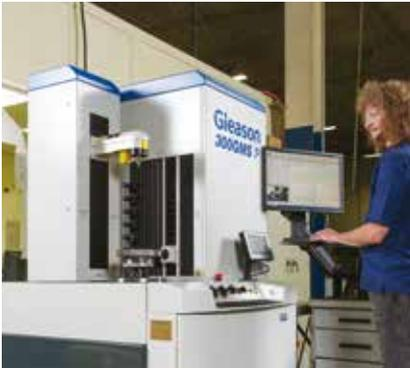
Machine operators now perform setup and in-process part inspections independent of the quality lab, saving precious time. The 300GMS®P is essentially part of the grinding cells, so the machine operators can perform in-process inspection, check charts and make machine adjustments on the fly.
